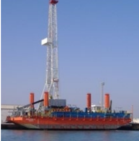
shallow water drilling unit (SEP)
