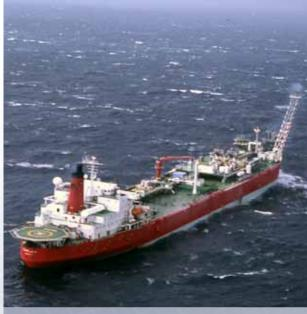
Lundin Petroleum as operator develops the Oudna oil field with a single subsea producer tied back to a FPSO. First oil November 2006 with a start-up production of 20,000 bopd. Estimated reserves are 12 MMB oil
