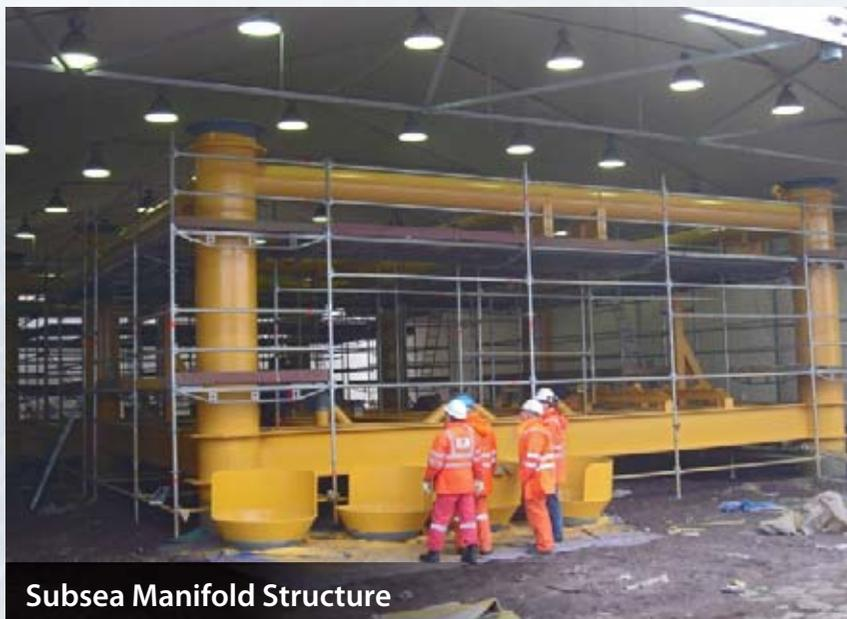
Subsea Manifold Structure
