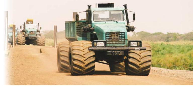
Seismic acquisition vehicles
